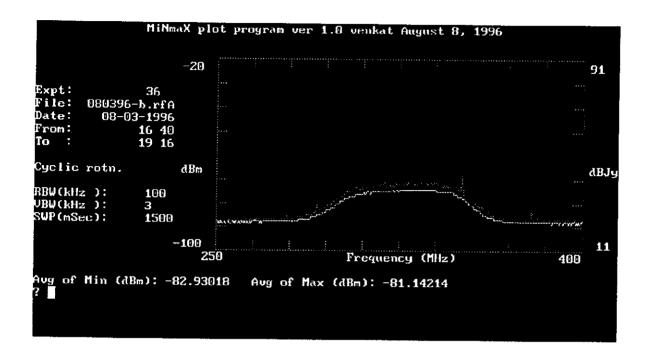
(d) 510 - 675 MHz band: As was explained in Annexure 5, the single RFI line at 636 MHz, which lasted for about 1.3% of the duration of the experiment spoiled the near-ideal picture in this band!
