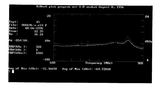
(f) 900 - 1400 MHz band: It should be remembered that the result seen below is with the spectrum analyzer in Peak-hold mode while the rest of the plots in Annexure 9 are in avaraging mode. I would not be surprised if many of the apparant lines seen below and also the relatively large difference between minimum and maximum are due to short-interval spikes at the site and will disappear if the recording is repeated in averaging mode.
