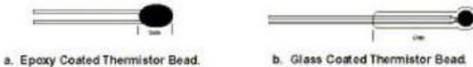
Figure 4 Thermistor element styles [2, p.24]
