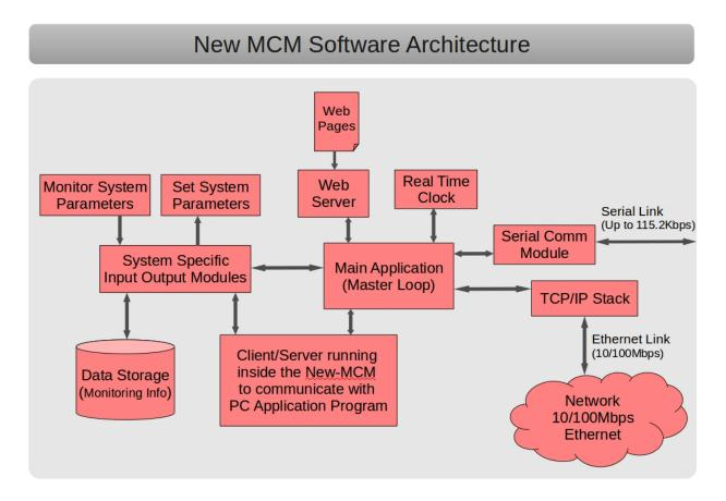
Software architecture of New MCM supports the Communication over the Ethernet as well as Serial link, 64 channel monitoring, 32 bit controlling, up to 1Gb data storage using FAT-16 file system. Furthermore, it will have Real Time Clock and Web server running inside.
