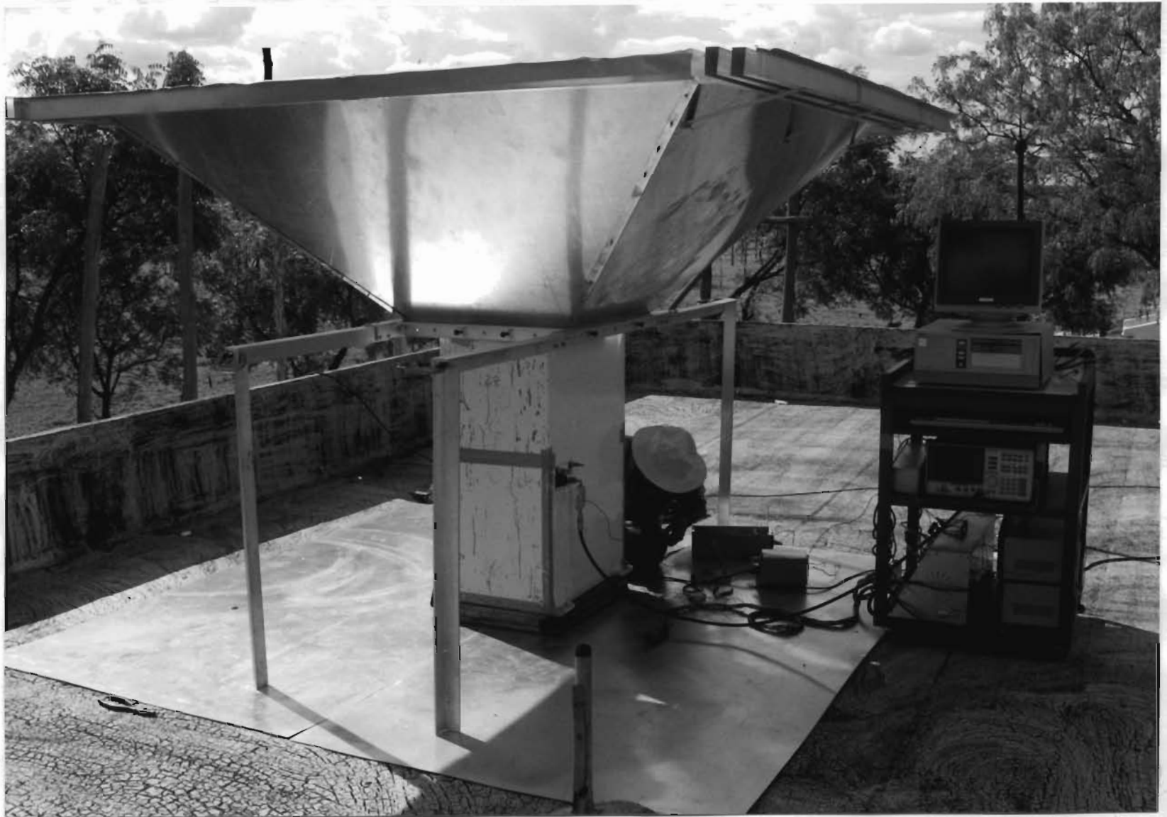
Photographic view of the Experimental setup for the measurement of the Cosmic Microwave Background Temperature
