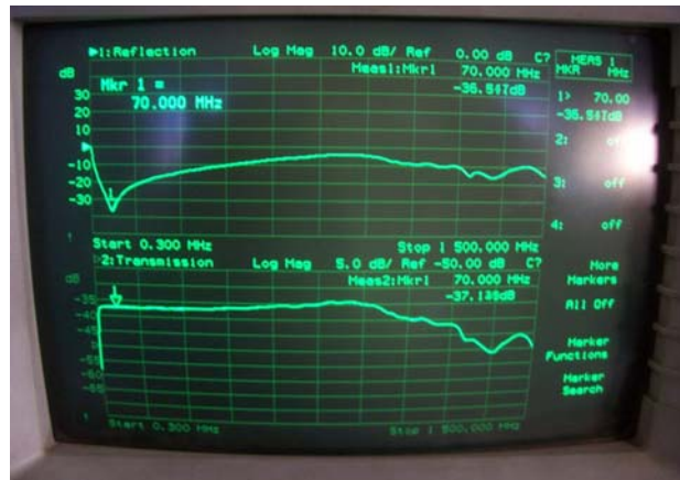
Figure 7.8(e): Frequency Response of S_{11} and S_{21}
