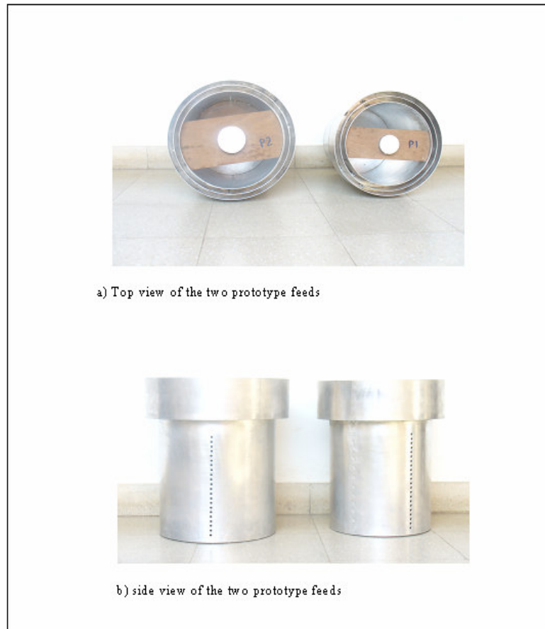
Fig 8.6 The two prototypes of the 700 MHz coaxial feed
