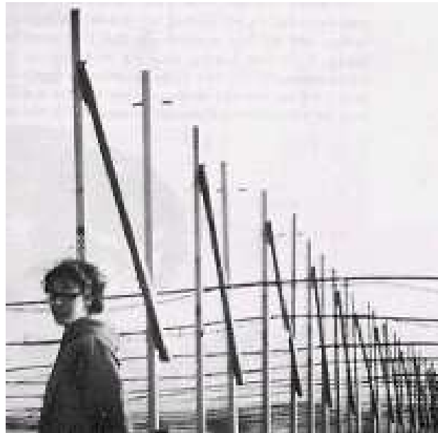
Figure 1.2: Mullard Radio Astronomy Observatory array (rectangular array containing 2048 dipoles operating at 81.5 MHz) used for the discovery of the pulsars in 1967 by Anthony Hewish and Jocelyn Bell (Hewish et al. , 1968). PSR B1919+21 is the first pulsar discovered by them. (Credit: http://www.mrao.cam.ac.uk/outreach/pulsars.html )
