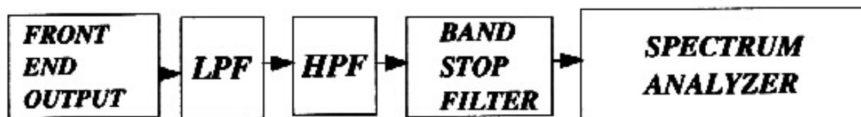
Fig 8. Block diagram of testing
