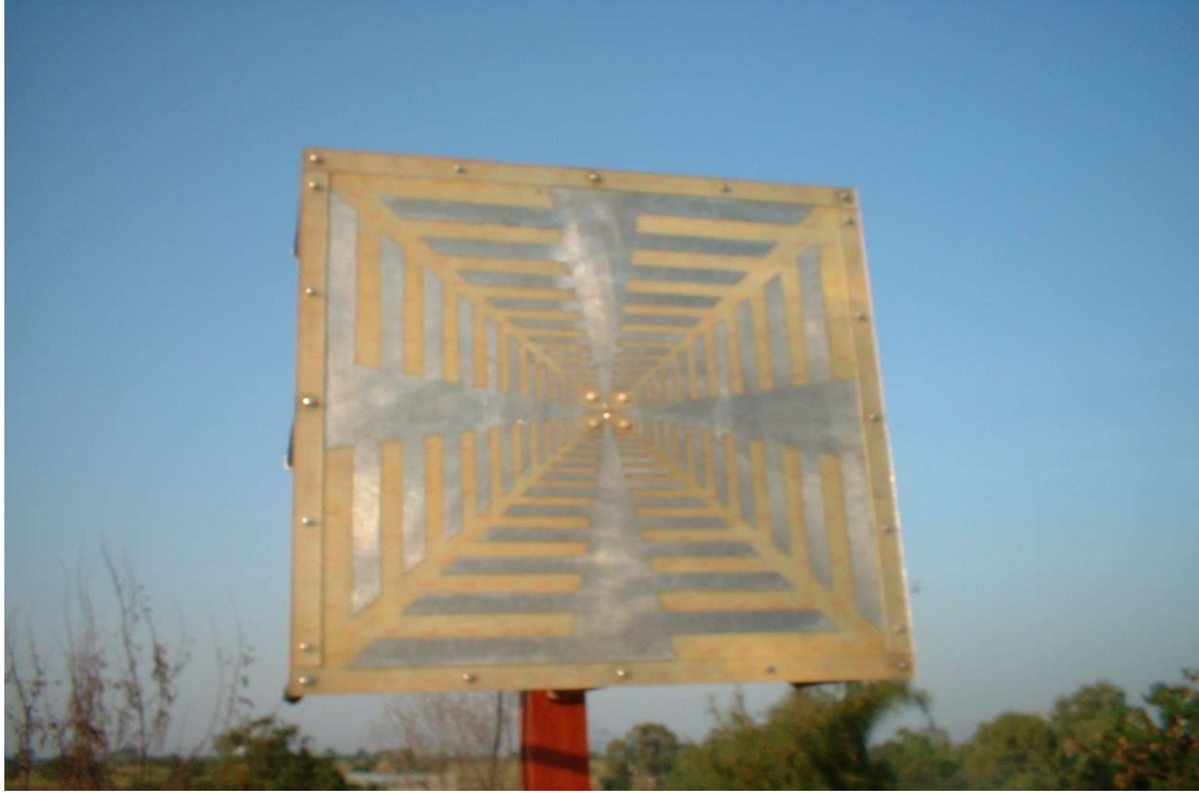
Fig. 10 Front View of the Antenna Mounted for Testing
