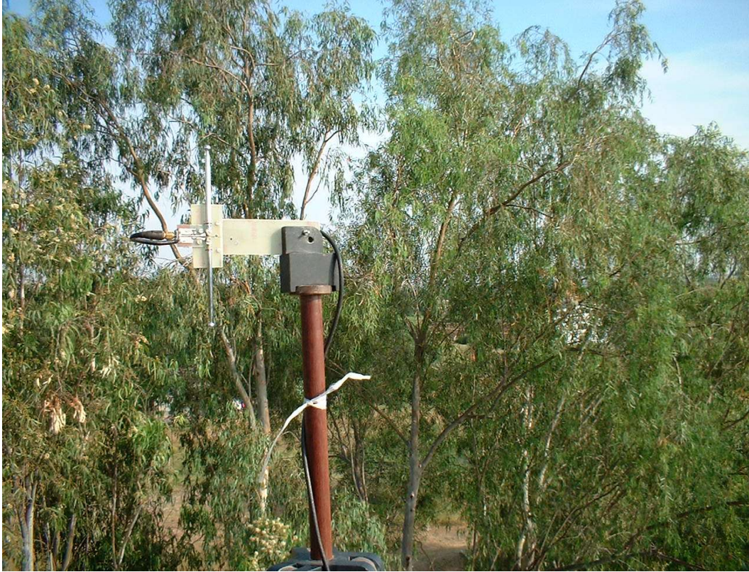
Fig. 9 The radiating dipole used in the experiment
