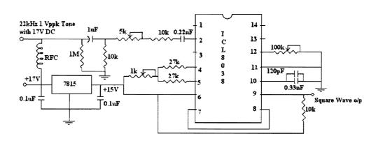
Though this circuit gives exactly the same signal and DC voltage as measured in the LNB cable, but when connected to LNB, circuit was unable to control LNB. This may be loading caused by impedance mismatch, and o/p stage of this circuit must be designed for 750hm. Additional effort to understand and solve the problem could not be put because of time constraints.
