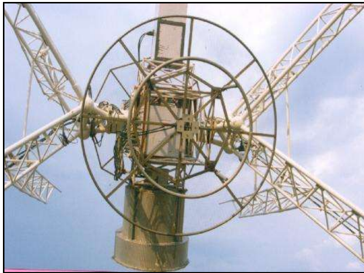
Fig-2: The four feeds mounted on the rotating turret
