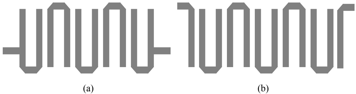
Figure 4.1: (a) tapped line input 5-pole Hairpin Filter (b) coupled line input 5-pole Hairpin Filter
