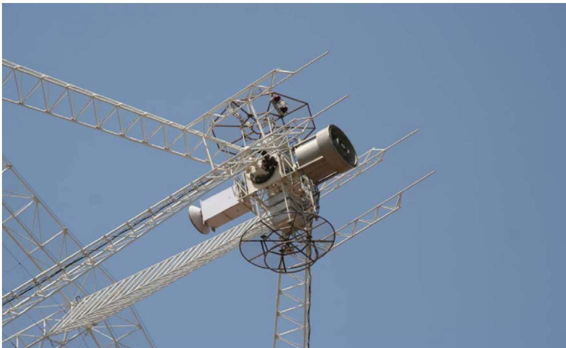
Fig shows the feeds mounted on the turret (GMRT)
