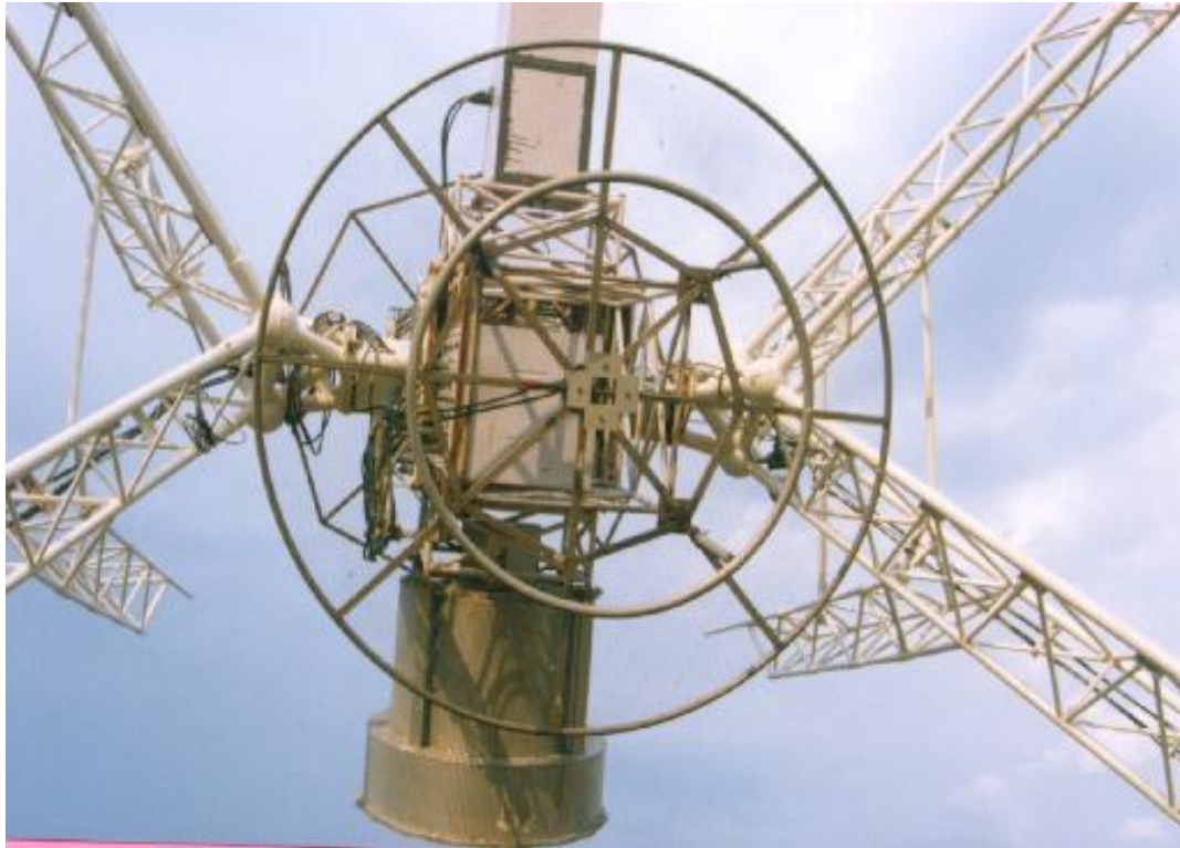
Fig:Four Feeds of one of the 30 antennas
