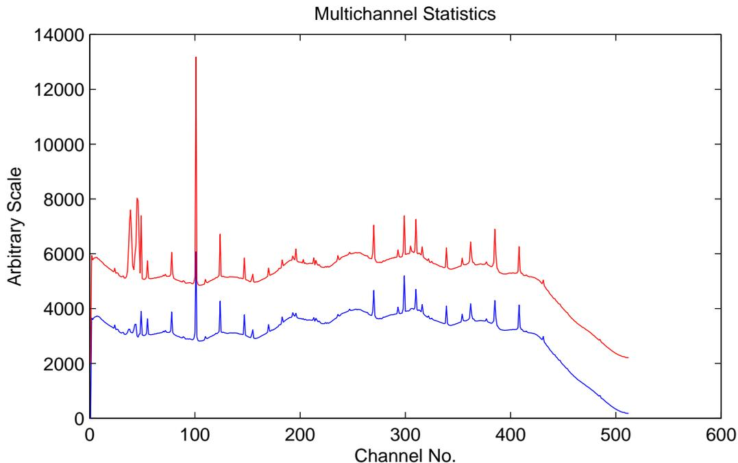
Figure 4.3: Statistics of multichannel data : mean and standard deviation across channels, superimposed on each other. Means are shown in the lower graph, and the standard deviations in upper one. The scaling is arbitrary. The plot is to show how both mean and standard deviation shoot up interference filled channels.
