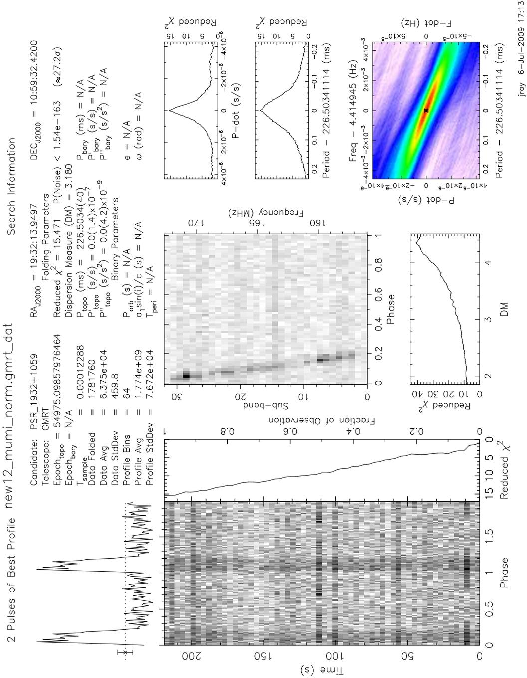
Figure 5.5: Folded profile of Multichannel - Multichannel data, collapsed at pulsar dm (3.18) and folded at pulsar period (226.5ms)
