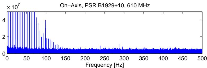
Figure 5.7: Fourier plot of On-Axis data, 610 Mhz, collapsed at zero dm
