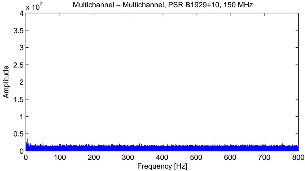
Figure 5.4: Fourier domain plot of Multichannel - Multichannel data, collapsed at zero dm
