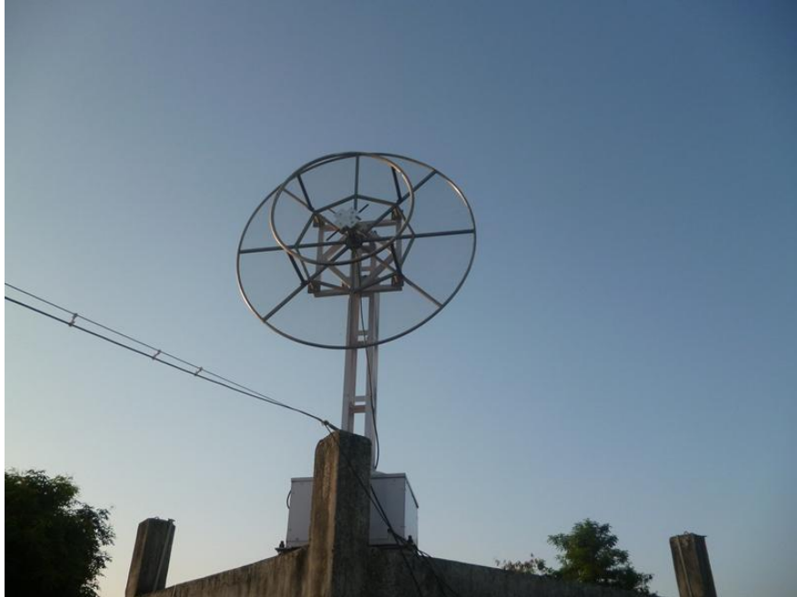
Figure Error! No text of specified style in document.-2 Modified Kildal feed
