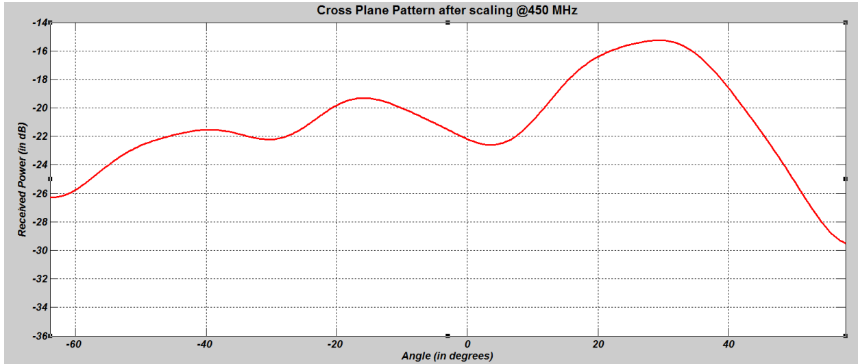
Figure 3-36 Cross Plane Pattern of Conical Dipole feed @ 450MHz
