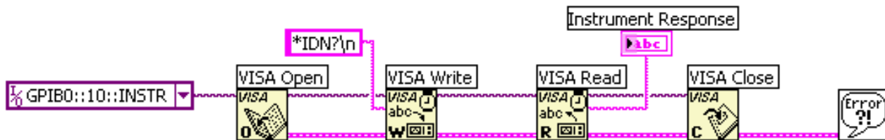
Fig 4: Control flow of a typical VISA application
