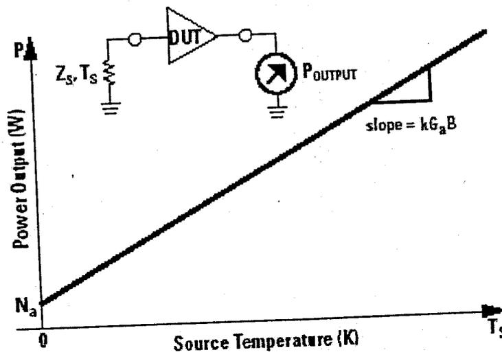
Figure 4.2: Noise Power vs Source Temperature Characteristic of Linear two port Devices
