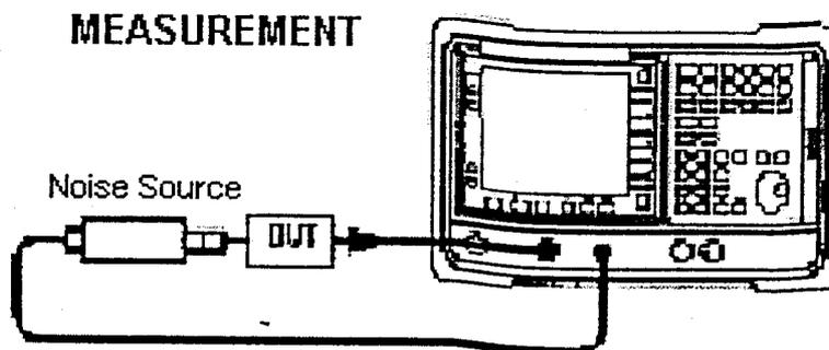
Figure 10.1: Amplifier Measurement Setup
