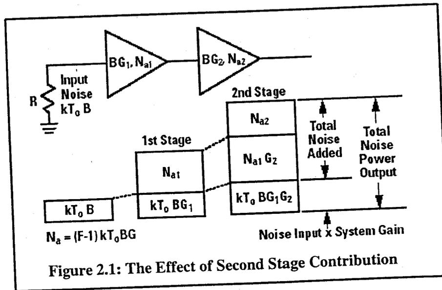
From Figure 2.1, the output noise will consist of source noise,  $kT_0B$  amplified by both gains,  $G_1G_2$ , plus the first amplifier output noise,  $N_{a1}$ , amplified by the second gain,  $G_2$ , plus the second amplifiers output noise,  $N_{a2}$ . The output noise can be expressed in terms of Noise Factor,  $F$  as
