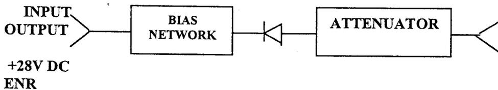
Figure 7.1: Block diagram of a typical Solid-State Noise Source
