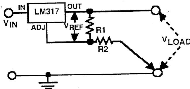
$$V_{LOAD} = V_{REF} \frac{(R_1 + R_2)}{R_1}$$
