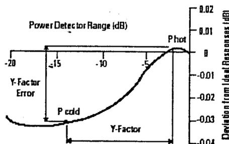
Figure 11.3: Non-Linear Behavior of Noise figure Meter
