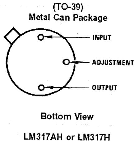
Figure 7.3: LM317 Connection Diagram
