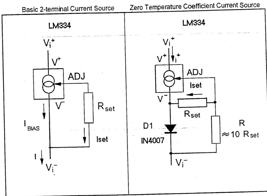
Figure 7.4: Zero Temperature Co-efficient constant Current Source
