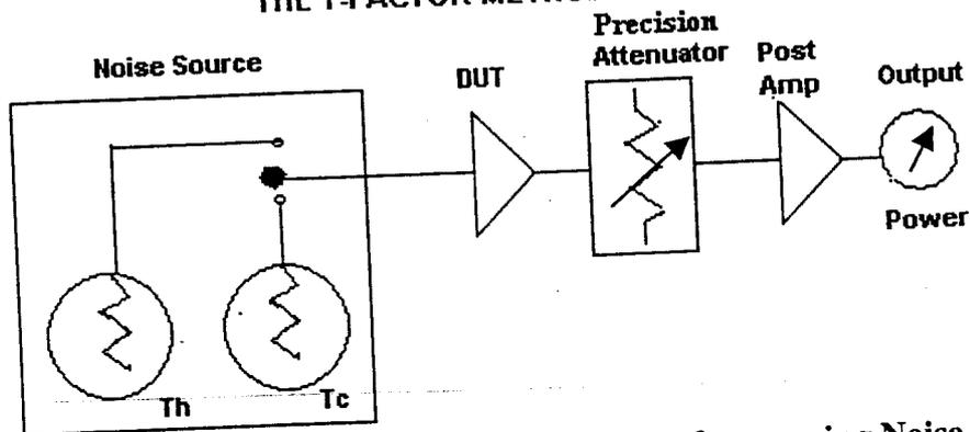
Figure 4.3: The schematic of the Y-Factor method of measuring Noise Figure
