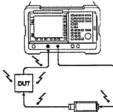
**Figure 11.1:** Spurious noise entering the test setup from external devices or connected components. Choosing a measurement instrument with good shielding is critical for NF measurements, since DUTs are often connected directly to the instrument. Well-designed instruments will exhibit very low emissions in the near field.
