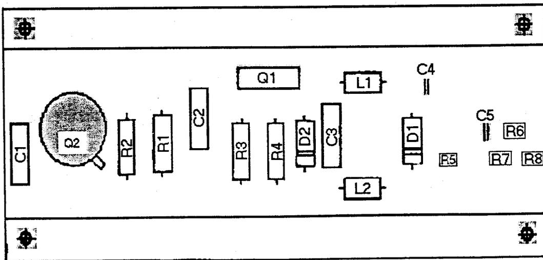
Figure 8.3: PCB Layout Viewing Silk Screen
