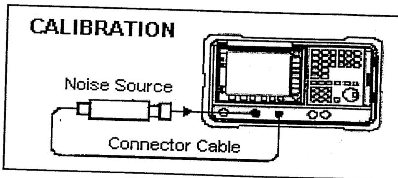
Figure 9.1: Noise Source Calibration Setup
