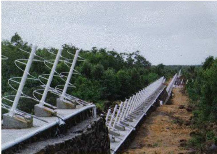
Figure 3.2: The Mauritius Radio Telescope. This is a low frequency (150 MHz) array of which the individual elements are helical antennas.
