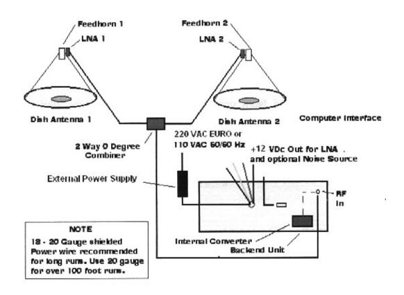
Figure 2. Interferometer Setup
