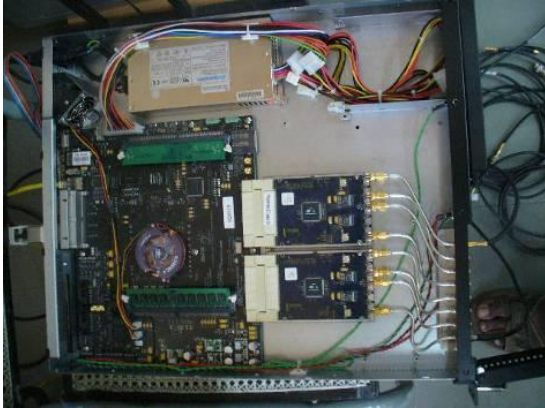
The CASPER based single board correlator in the lab test set-up
