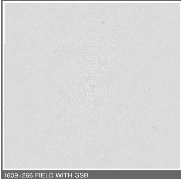
A first light image from the GSB : radio intensity map of the region of the sky around the source 1609+266, at 1280 MHz. Beside the central point source J1609+266 of 4.8 Jy, a few other sources, including a couple of double radio sources can be clearly seen. The dynamic range achieved in this image is 1.4 \times 10^5 . (Courtesy : Subhashis Roy)
