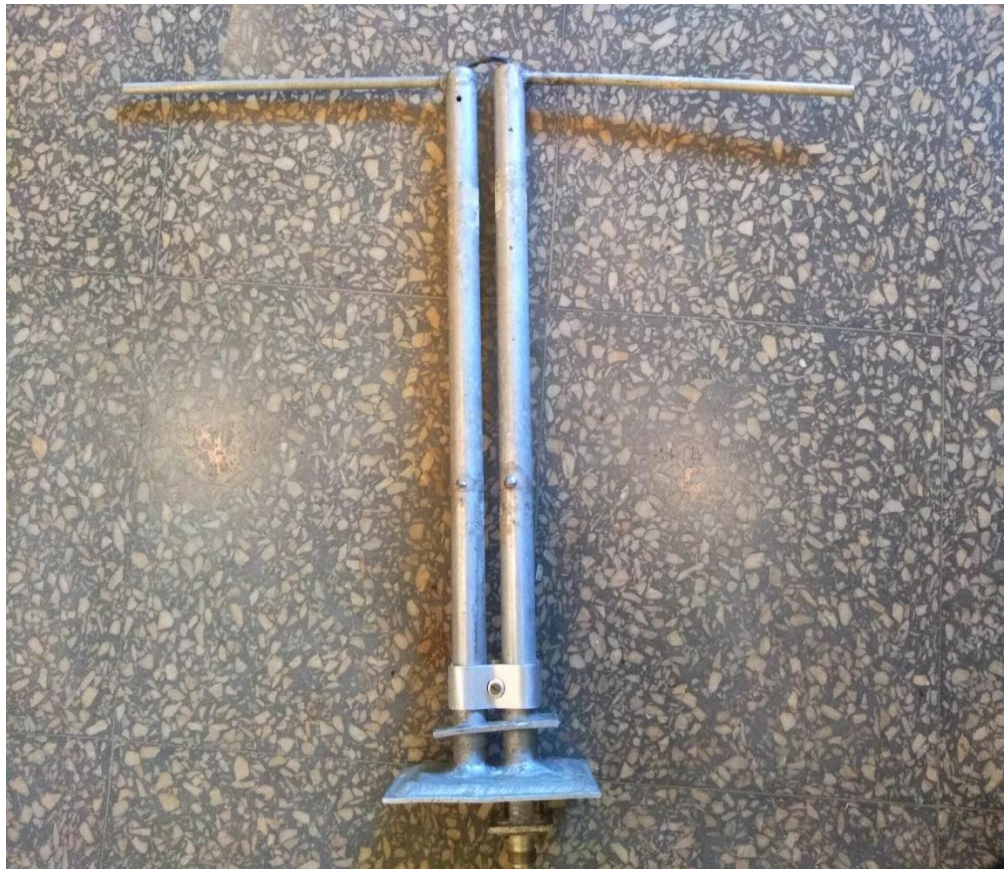
Figure 1.1: Dipole antenna used as transmitter (center frequency of dipole 326.5MHz)
