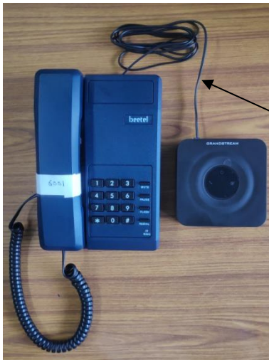
Image3&4: Grandstream make VOIP Adaptor + Phone with aluminium shielded enclosure
