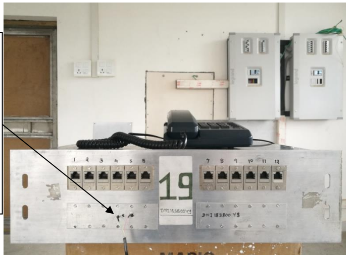
Image3&4: Grandstream make VOIP Adaptor + Phone with aluminium shielded enclosure
