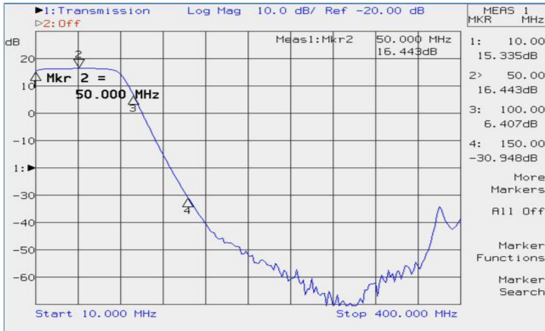
Fig 6.3.1: BB IN to BB OUT Frequency response @ 100MHz Low Pass Filter Selection (Input:-30dBm)
