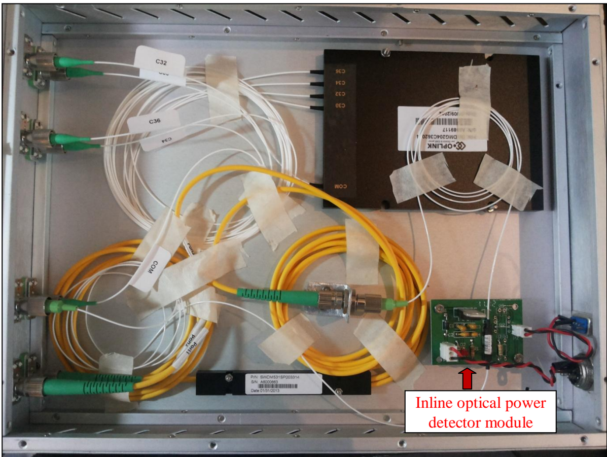
Figure 7. Optical De-Multiplexer with optical power detector unit
