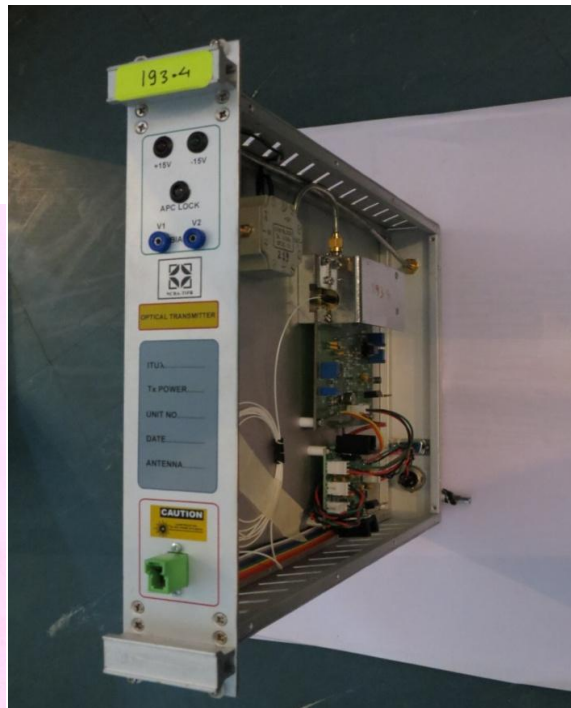
Figure 8. Populated Optical Transmitter Board
