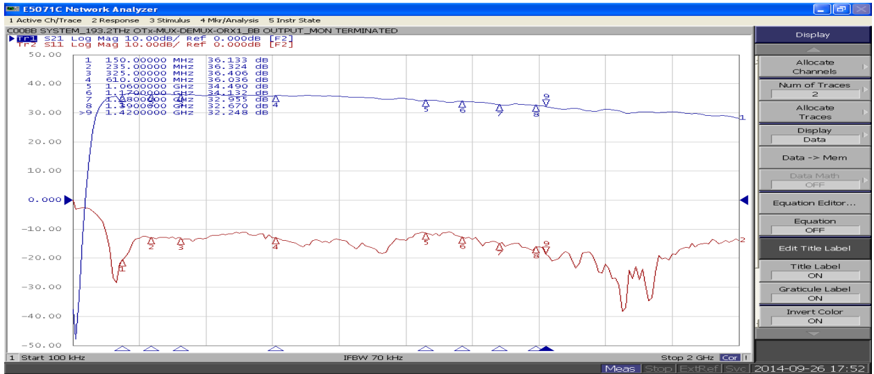
Figure 16. Response of cascaded Broadband fiber optics system
