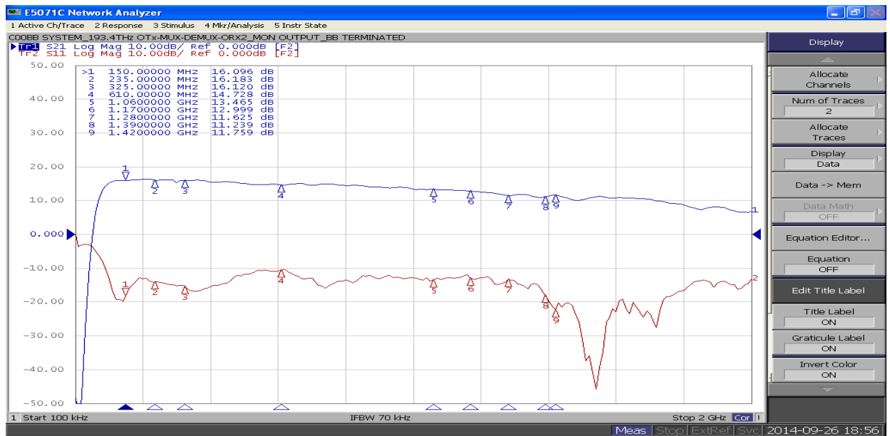
Figure 16. Response of cascaded Broadband fiber optics system
